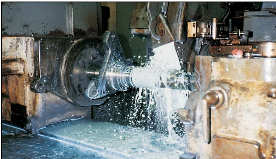
THIS MACHINE CAN HANDLE UP TO A 14" DIAMETER SHAFT 50" LONG.
